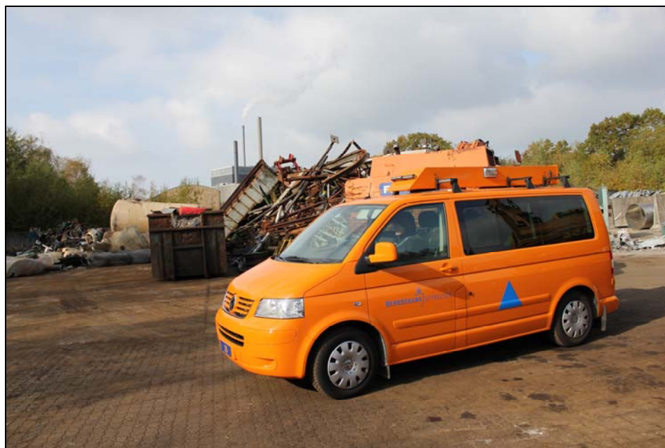
Figure 13. Car-mounted mobile 1028-channel gamma multichannel analyser system equipped with a 4L NaI(Tl) detector, position logger and automated alarm features.
